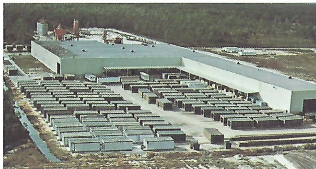
MODULAR CONSTRUCTION: The first two hotels at Walt Disney World will feature guest rooms of lightweight modular steel construction. Fabricated in an on-site assembly plant (left), the rooms are trucked to the construction area, where they are lifted into place and utilities are plugged in.
